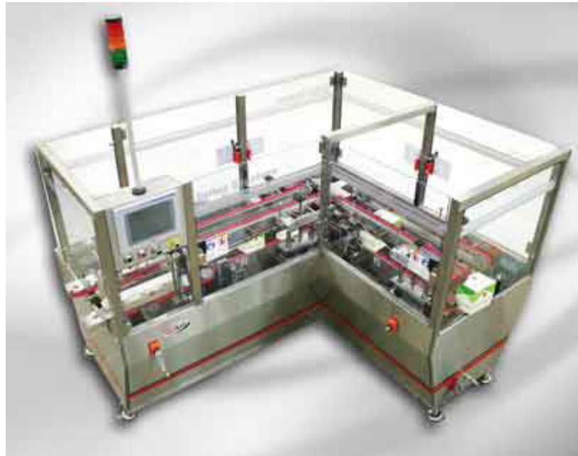
Delkor Capstone Carton Closer with Intelligent Positioning™ Technology
