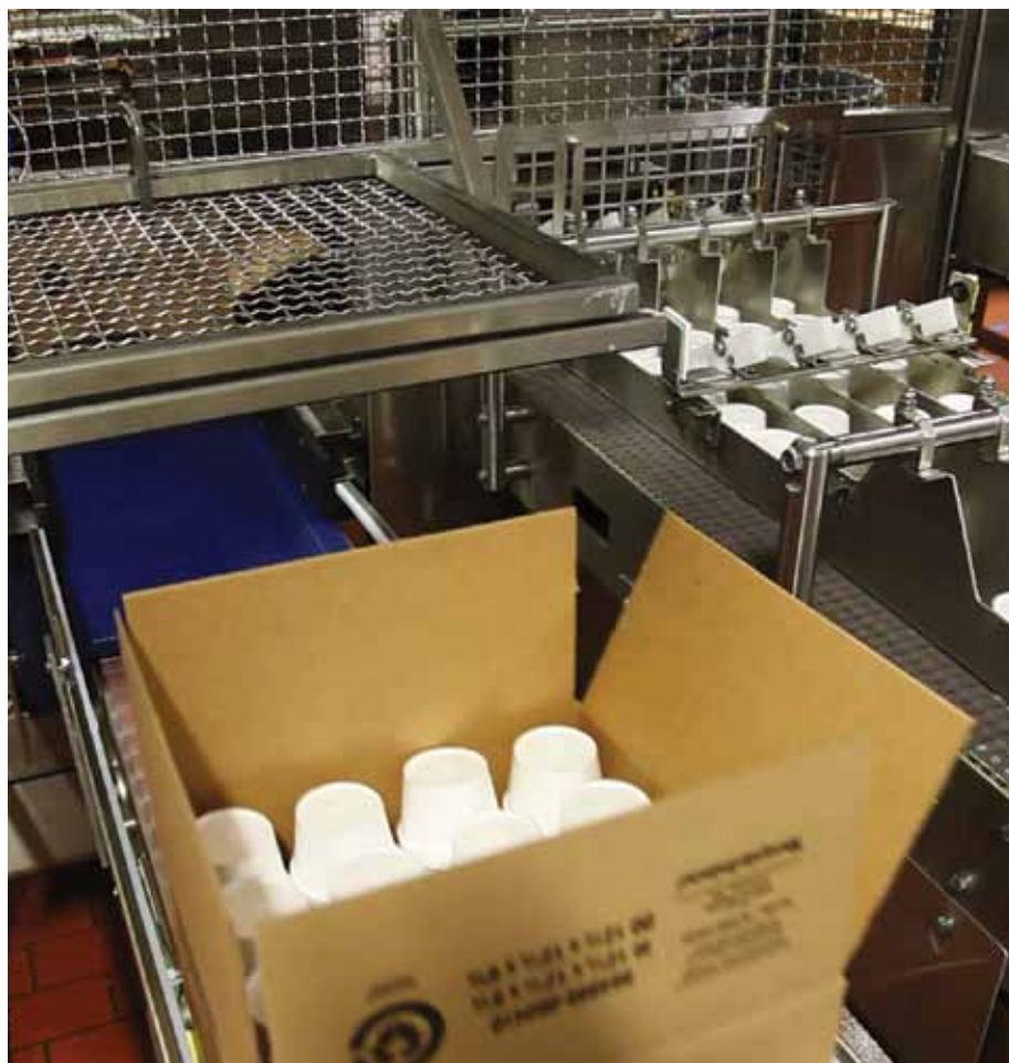
To make efficient use of floor space, a case taper is integrated into the case packer
